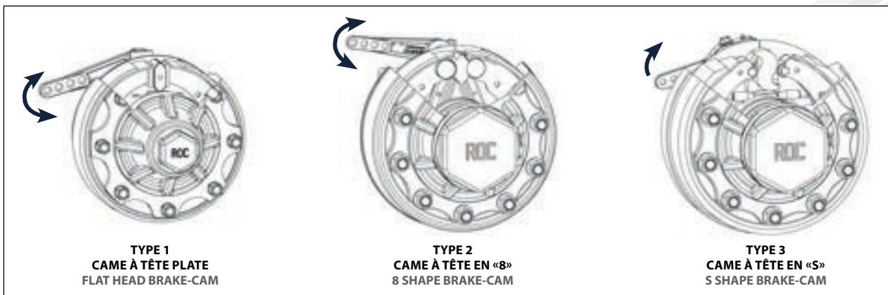
↗ Sens de rotation de la came / Direction of rotation of the cam
